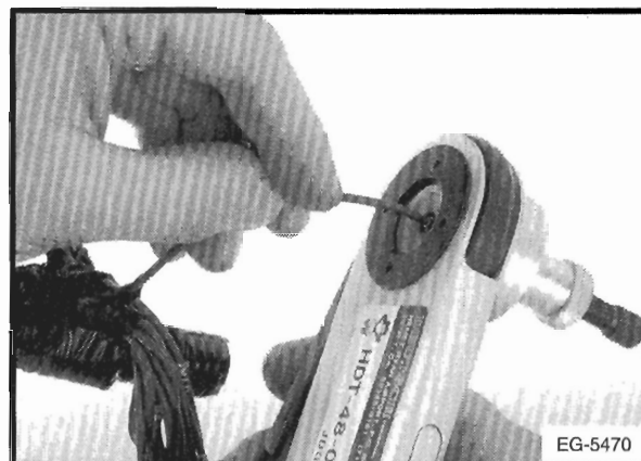
Figure 6-8. – Contact Crimping
